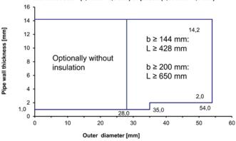
L measured from the surface of the penetration seal (see ANNEX B-1 to C-2 of the ETA).
