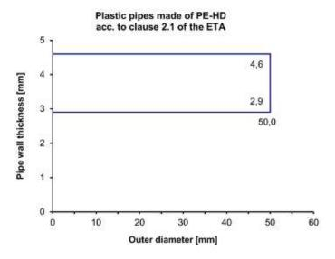
Interpolation between pipe diameters and wall thicknesses for plastic pipes according to clause 2.1 of the ETA in flexible walls, rigid walls and rigid floors - mixed penetration seal
