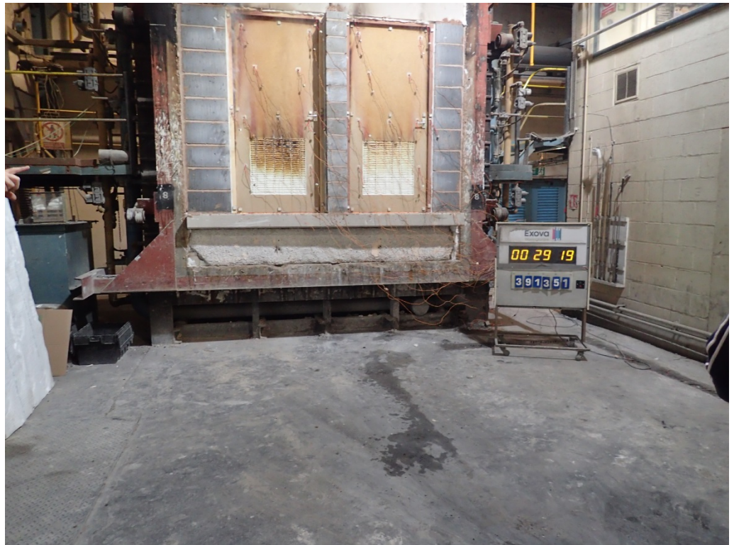
The unexposed face of the doorsets after 29 minutes of testing
