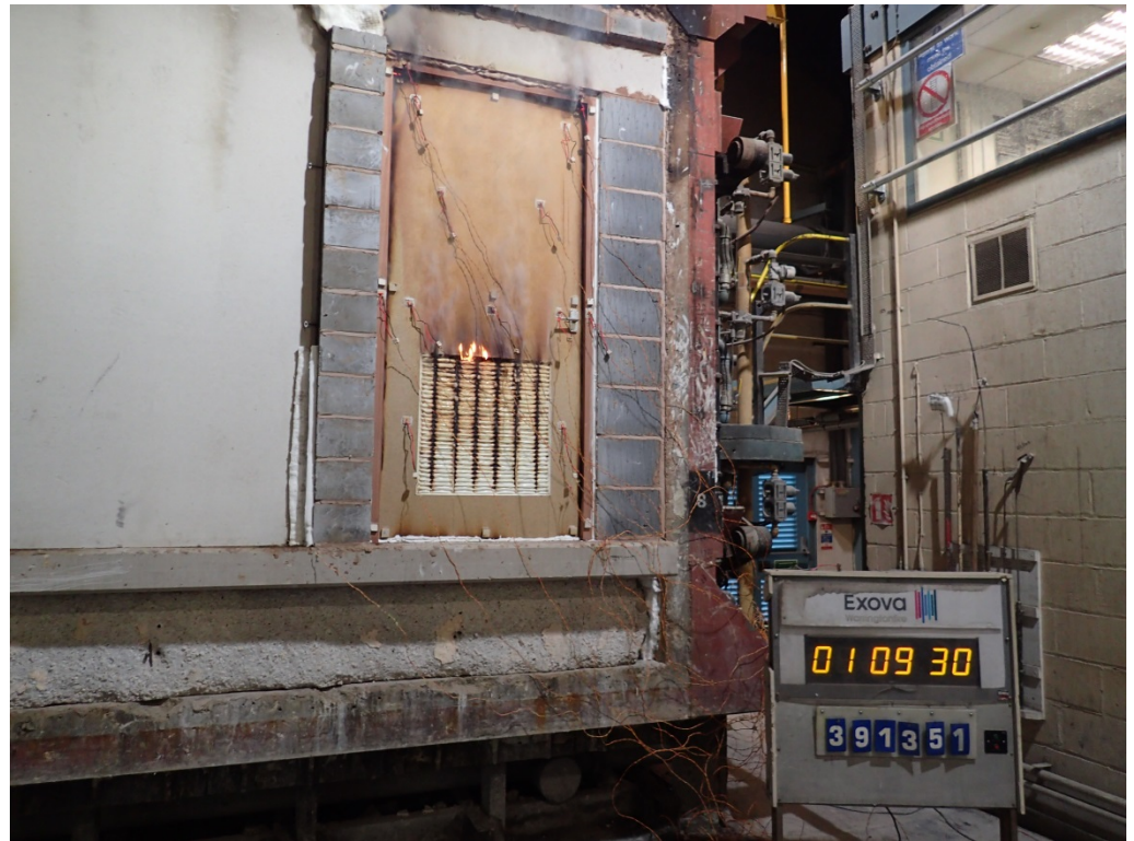
Flaming seen from the top of the grille on Doorset B after 69 minutes of testing
