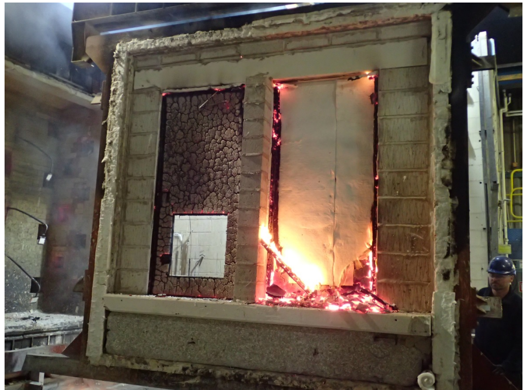
The exposed face of the doorsets immediately after the test
