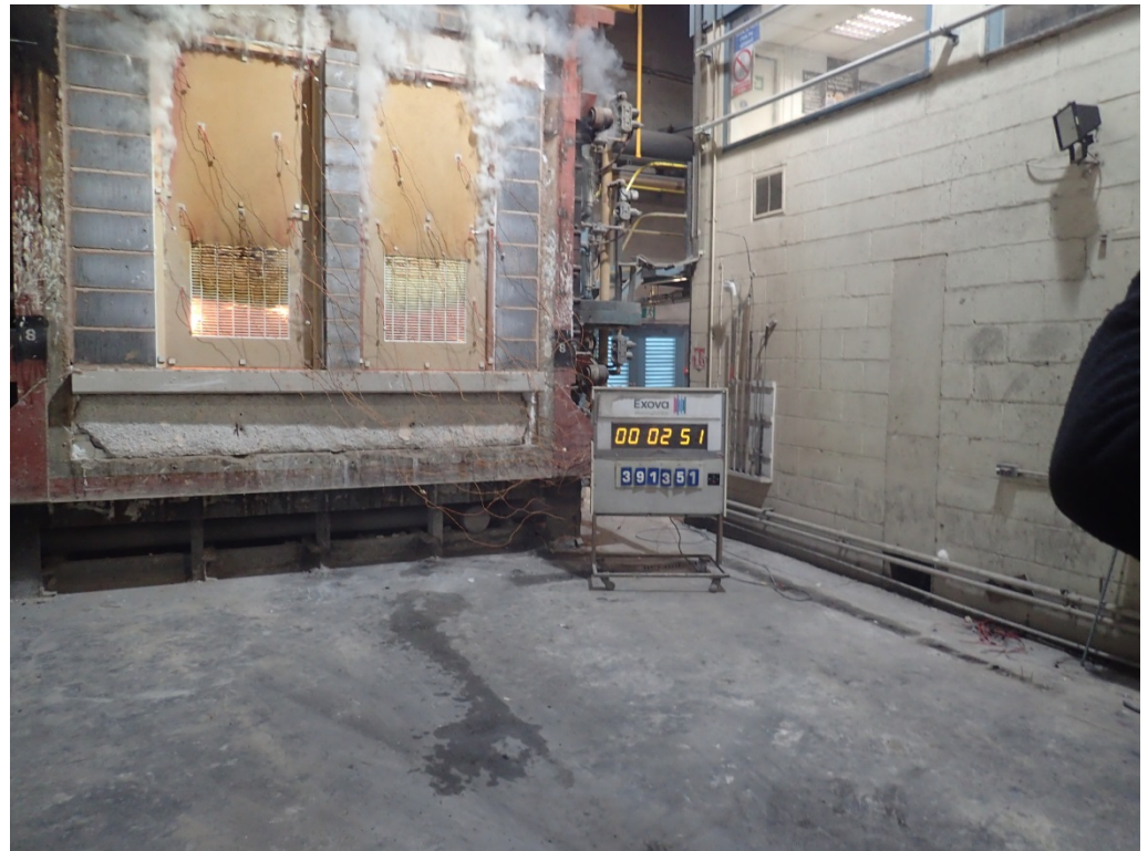
The unexposed face of the doorsets after 2 minutes of testing
