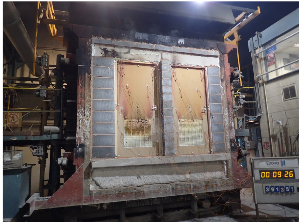
The unexposed face of the doorsets after 9 minutes of testing
