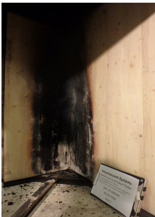
Photographs 3 and 4: Specimen 1 after testing
