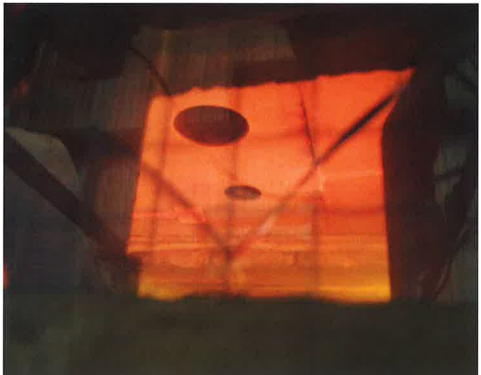
The exposed face of the ceiling after a test duration of 30 minutes
