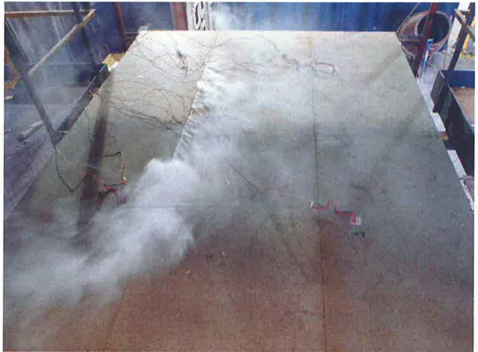
The unexposed face of the ceiling after a test duration of 90 minutes
