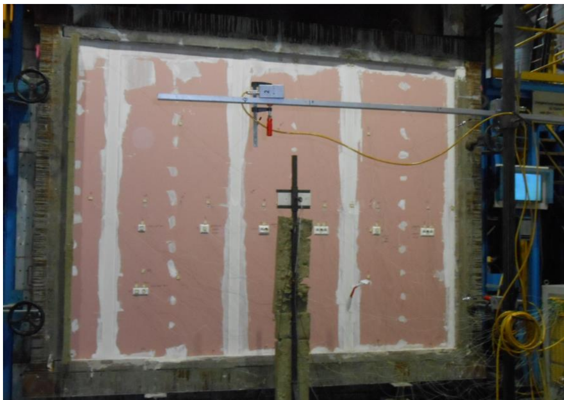
Photo 3 Hollow wall boxes installed in wall at the non-exposed side (NS)
