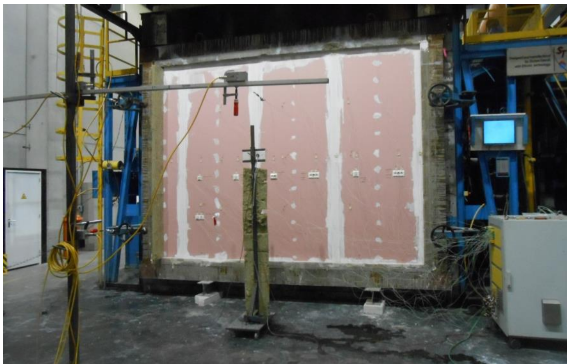
Photo 18. Test specimen before test, fire side
