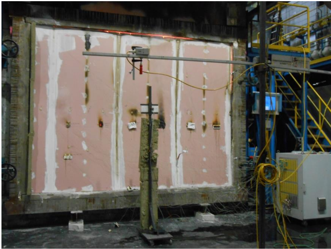
Photo 22. Test specimen after 136 minutes of heating
