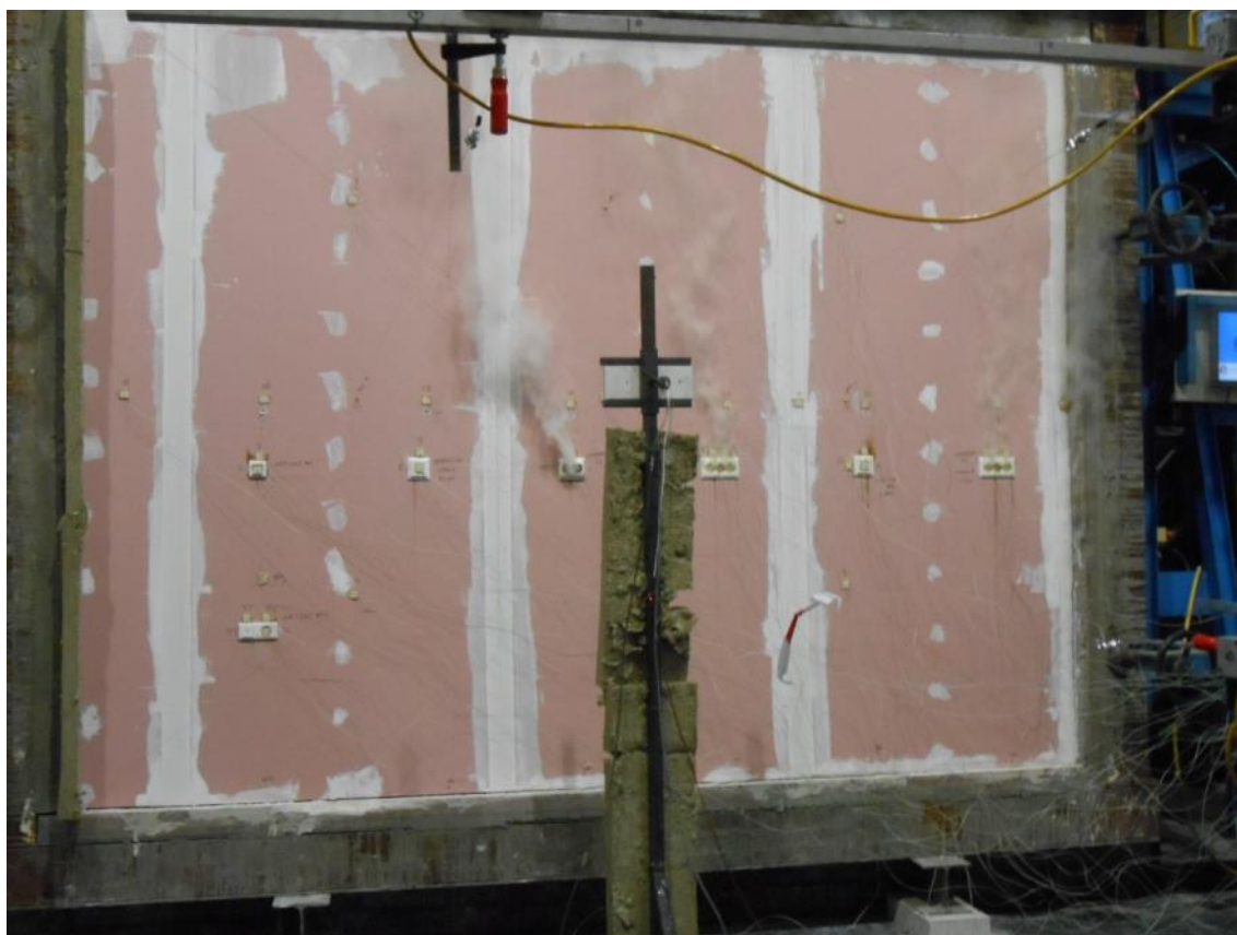
Photo 20. Test specimen after 66 minutes of heating
