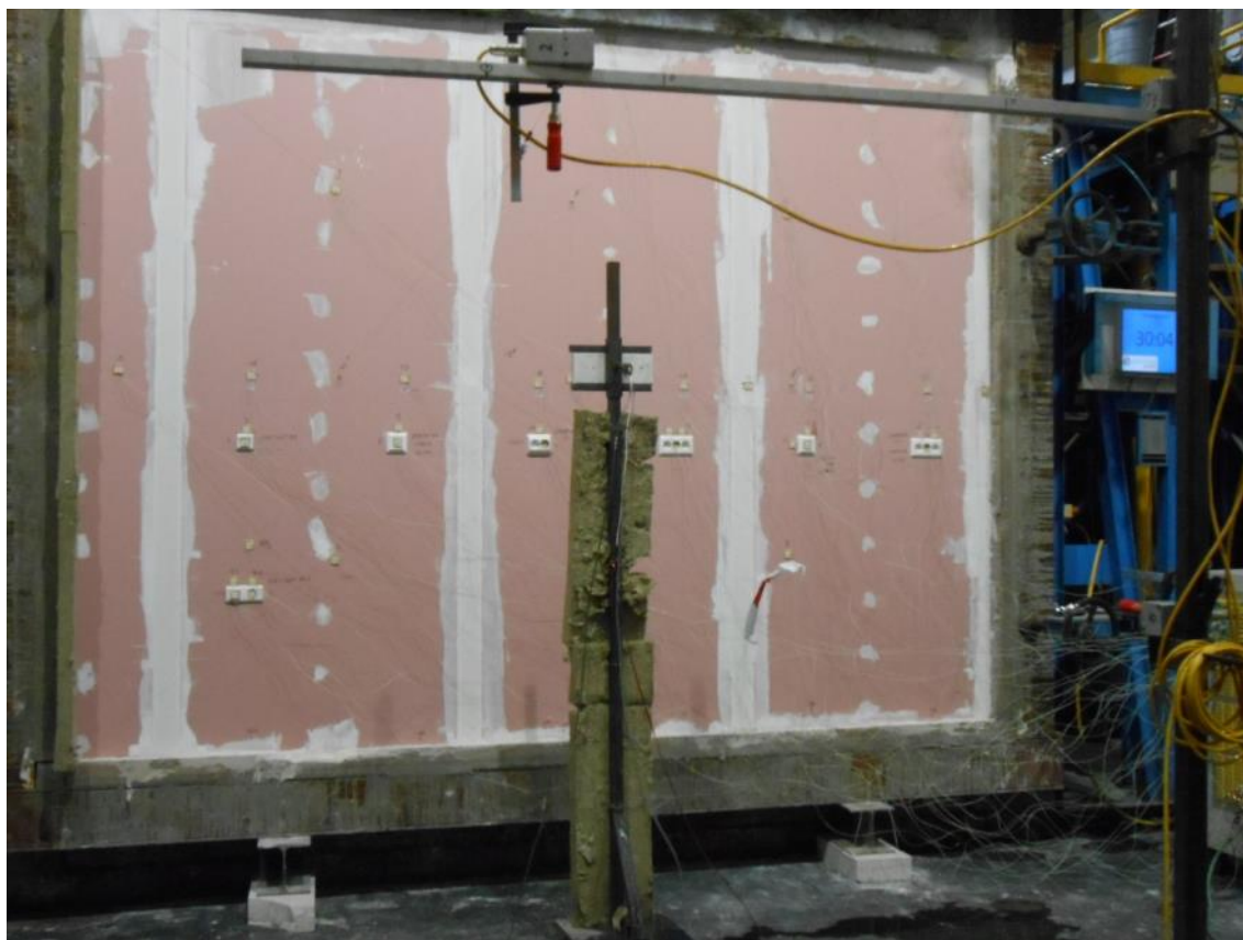
Photo 19. Test specimen after 30 minutes of heating
