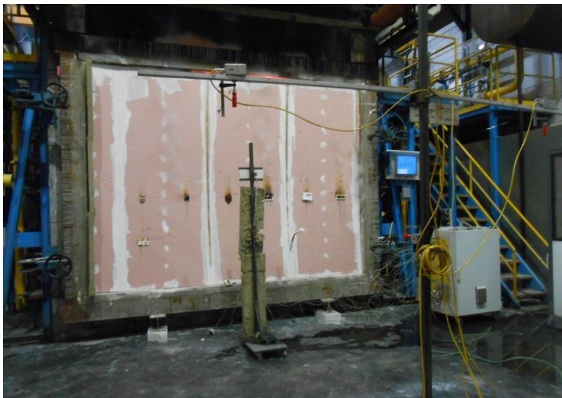
Photo 21. Test specimen after 120 minutes of heating
