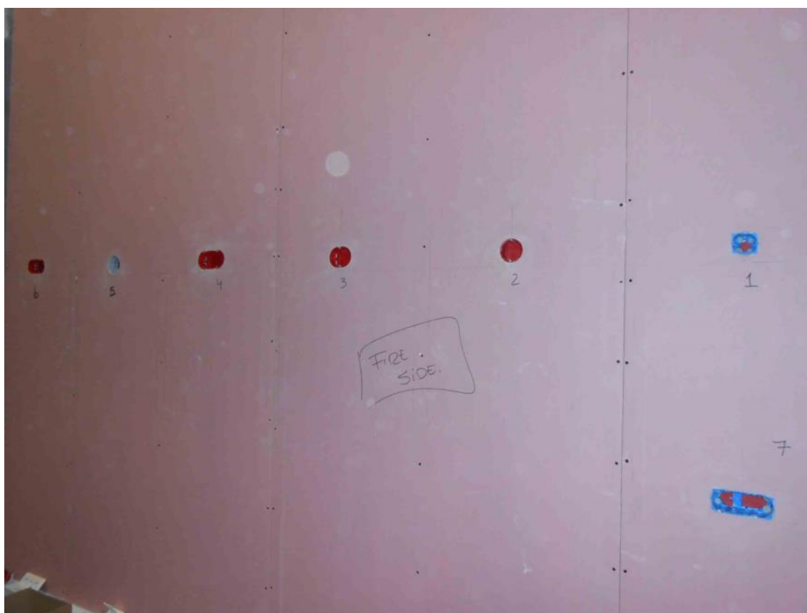
Photo 2 Hollow wall boxes installed in wall at the exposed side (ES)
